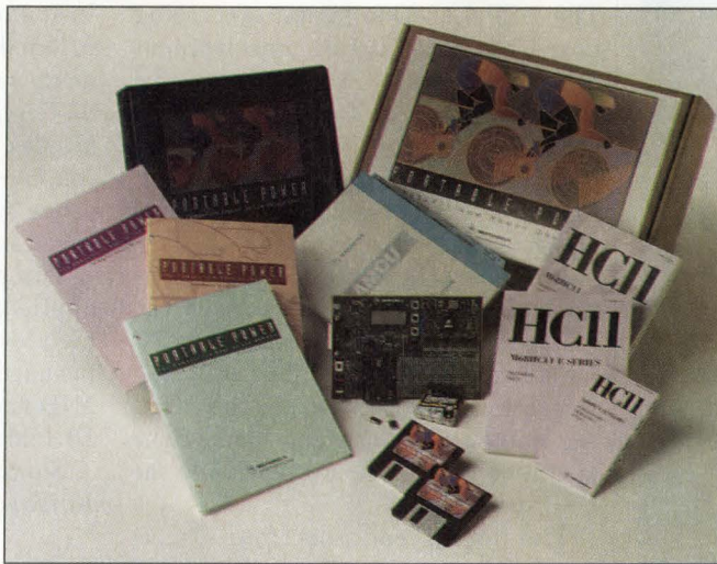
This evaluation kit allows you to learn more about low-power system design; you can play games with clock speeds, supply voltage, and code.
