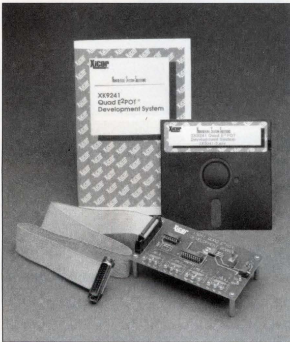
The XK9241 can be used in a production environment to optimize the settings of the E 2 POT.
