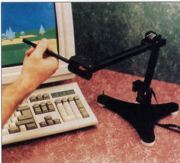
Immersion Probe provides 3-D position and orientation information to a computer via a serial port.
