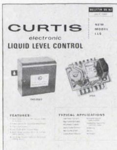
The Curtis LLS is a versatile, electronic static device incorporating a silicon-controlled rectifier (SCR) for operating the control relay. Operation is accomplished by sensing a minute current flowing between submerged probes. This AC current triggers the SCR and energizes the control relay. One set of control relay contacts allows internal pump-up or pump-down control, leaving two sets of contacts for the control operation function. Fully described and priced on new 2-page brochure DS-162.
