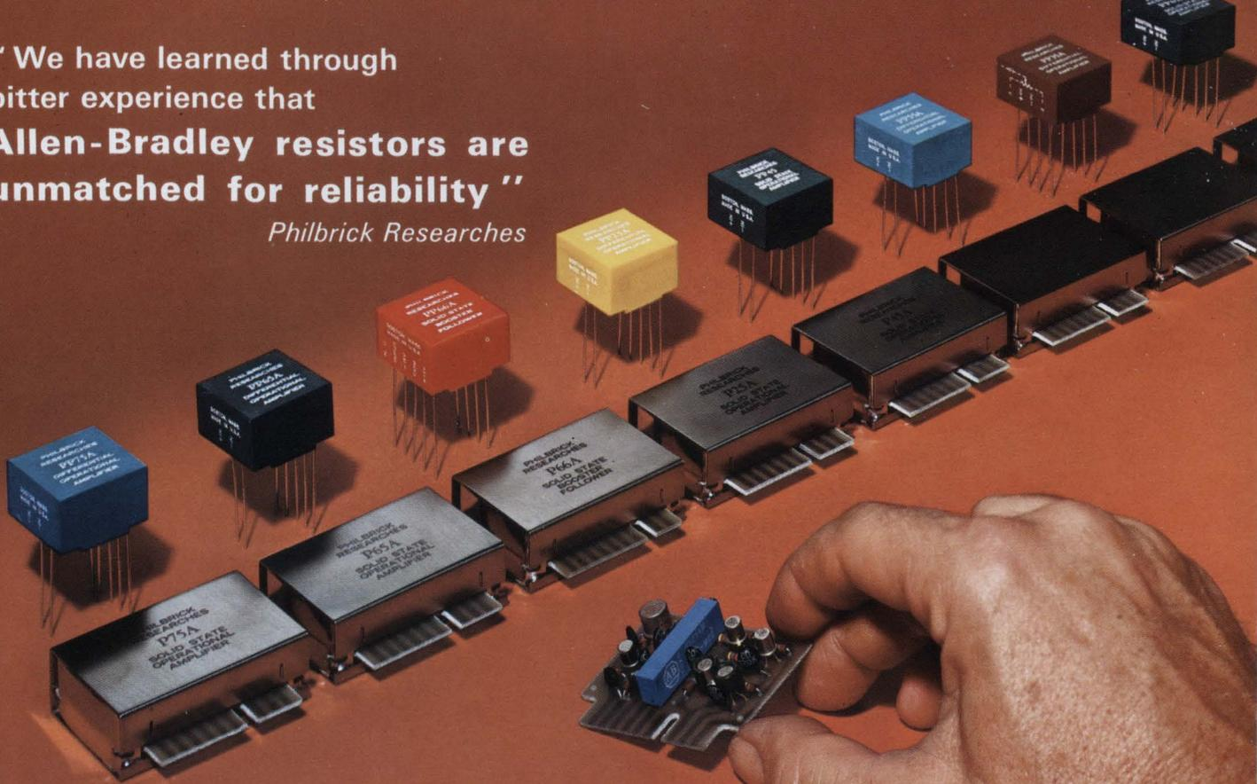
Typical Philbrick solid state operational amplifiers. The Model P65A differential operational amplifier with cover removed shows the use of Allen-Bradley Type N adjustable fixed resistors and an Allen-Bradley Type N adjustable fixed resistor for zero balance adjustment.
