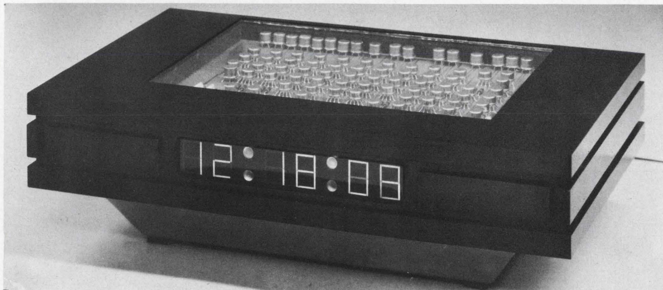
1. Digital clock built with 90 integrated circuits uses a 1-MHz oscillator as a basic timing source and achieves an
