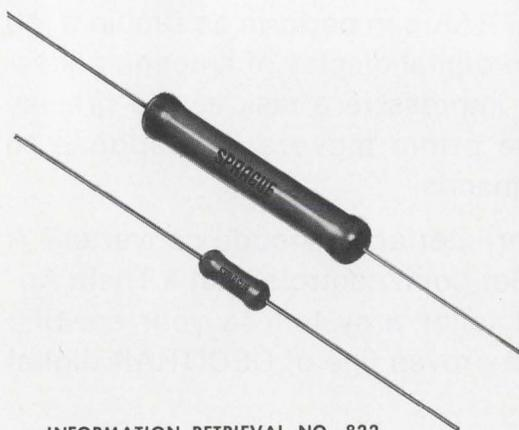
All-welded end-cap construction eliminates moisture along the leads, also anchors leads securely to resistor body. Expansion coefficients of vitreous enamel coating, ceramic core, and end caps are closely matched. Standard wattage ratings include 1, 2, 2.5, 3, 5, 7, 10, and 11 watts. Also available with radial tab terminals in ratings from 8 to 230 watts.
