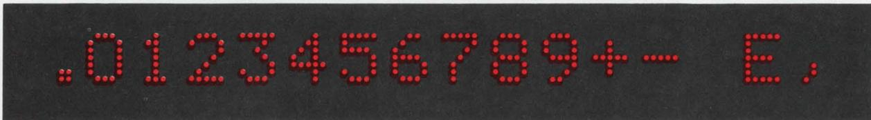
By utilizing the phenomena of preferential glow transfer and glow shifting, the initial glow caused by cathode ionization in the dot matrix may be moved through selected holes to a visible position on the top surface. A sequential flow of light is thus achieved without separate drivers for individual columns and rows.
