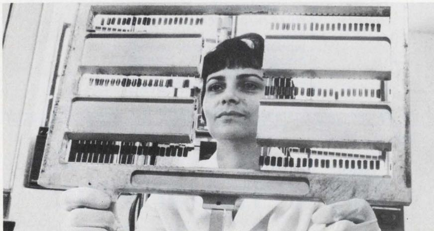
Solid-state rectifiers to replace tube components for color TV. Such devices eliminate sources of ionizing radiation.
