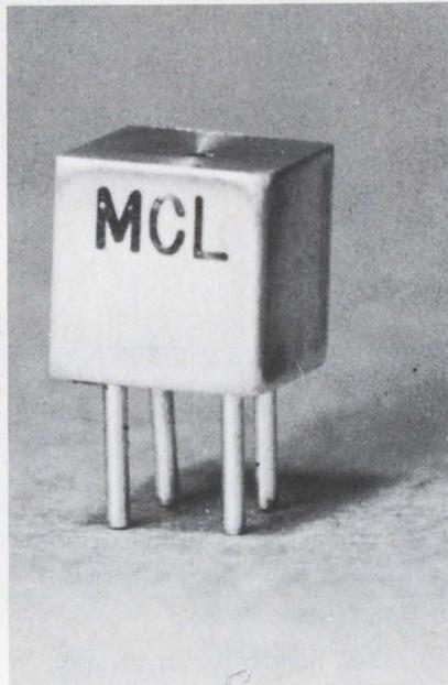
a new microminiature double-balanced mixer operates from 25 kHz to 500 MHz with a typical noise figure of less than 6 dB. This tiny device, model ASK-2, features a volume of only 0.05 cubic inches, occupying approximately the same board space as a TO-5 transistor package.
