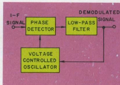
6. A phaselock loop can serve as a threshold extension fm modulator. Since the VCO is made to follow the i-f, its control voltage is the demodulated output.
