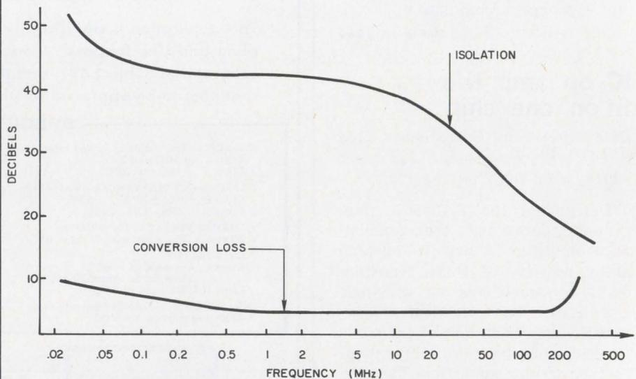
Minimizing conversion loss and maximizing isolation, a new transistor-sized double-balanced mixer spans the frequency band of 25 kHz to 500 MHz. Occupying but 0.05 cubic inches, this microminiature device holds conversion loss to 10 dB maximum and keeps isolation to 15 dB minimum.
