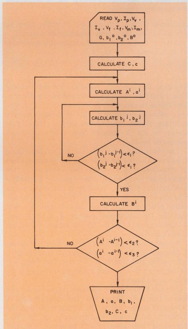
5. Flow chart of computer program shows the steps to be followed in determining parameters of the curve-fitting equation. Note the iteration steps for the  $a$ ,  $A$ , and  $B$  parameters.
