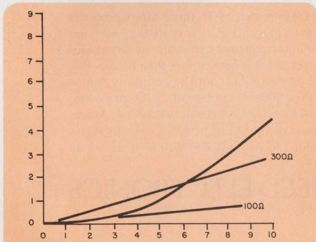
2. The nonlinearity of the #344 bulb is used to increase the negative feedback factor when the output increases. 100 Ω and 300 Ω lines are shown for reference.
