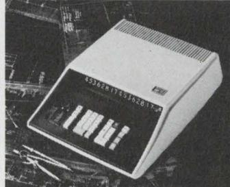
**6** Sharp MAXI. 16 digit capacity. Automatic drop-off. Pre-set or floating decimals. Dual decimal systems for memory and display. Automatic squaring. Round-off, up
