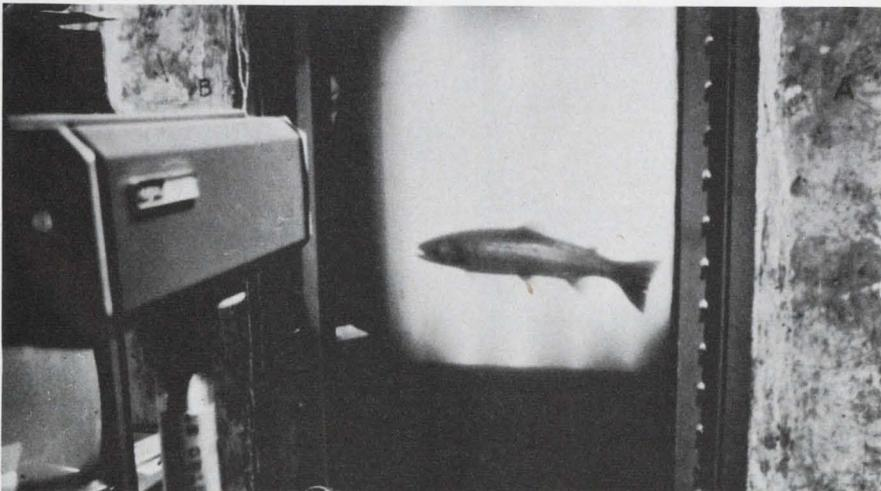
Salmon passes viewing window at the Willamette Falls, Ore., automatic counting station. A closed-circuit TV camera relays the picture to a video tape recorder later used in fish identification.
