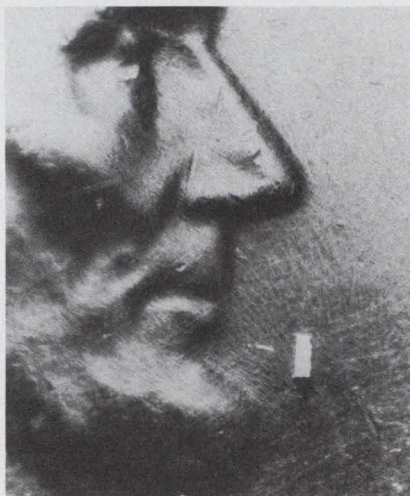
New semiconductor laser makes a penny look big. This is the first of its kind to run continuously at room temperature. The power source is no larger than a flashlight battery.
