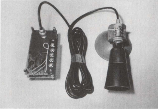
Passive ultrasonic "blind-spot" detector with directional horn.
