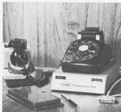
An unattended answering device, the Telanalysis 240, "answers" the telephone in a doctor's office, and an operator at the United Medical Laboratory—a large mail-order laboratory in Portland, Oregon—transmits the results of a lab analysis at any time of day or night to any part of the U.S. It rents for $15 per month.
