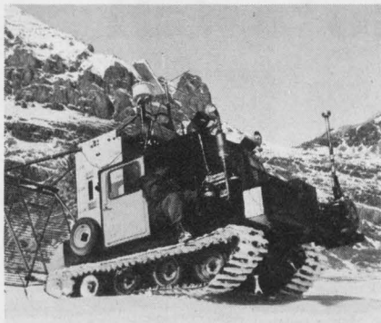
This snow cat carries a Ruggednova interfaced with two radar systems to help map the Canadian glacial fields.
