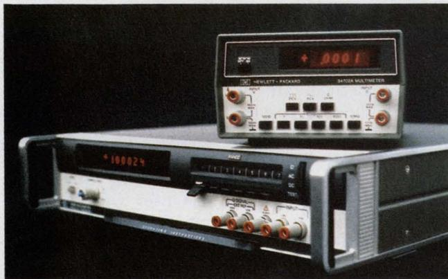
Hewlett-Packard offers its 3470—a plug-on series of interchangeable modules—and the self-testing 3490A.
