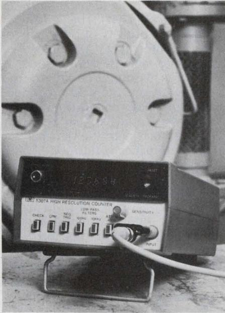
No need to set gate times or make adjustments—the new 5307A counter rapidly measures low frequency events.
