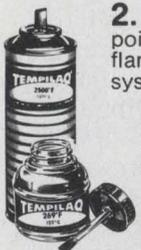
**2. TEMPILAQ<sup>®</sup>:** materials of calibrated melting points suspended in an inert, volatile non-flammable vehicle. Available in over 100 systematically spaced temperature ratings from 100° to 2500°F. Tempilaq<sup>®</sup> indicates its temperature rating by liquefying within  $\pm 1\%$  of its rating. Available in bottles or spray cans.
