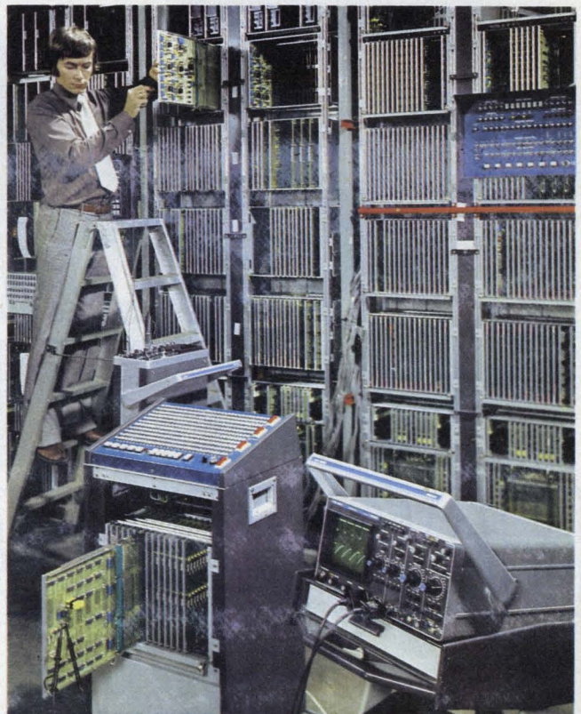
Dual-trace oscilloscope from Philips has a bandwidth of 120 MHz. Using a special power supply, the PM 3260 can operate from almost any line voltage and frequency. It consumes only 45 W and needs no fan for cooling.
