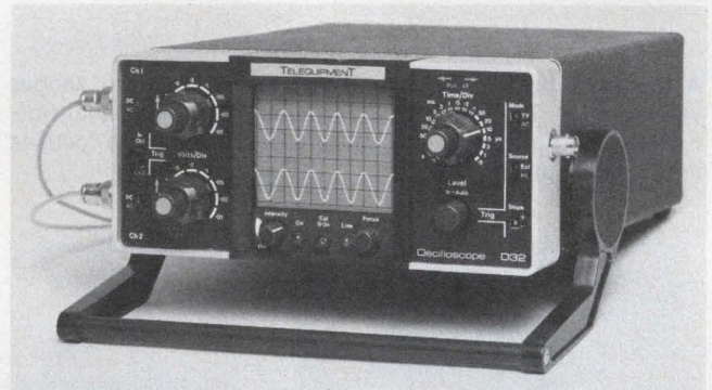
A miniature dual-trace scope that weighs only 10 lbs and has a bandwidth of 10 MHz is the D32 from Tektronix.
