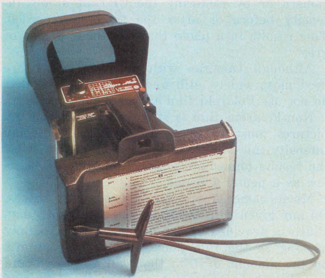
A portable scope camera that has a viewing hood to permit monitoring of the waveform on the CRT is the Model SC02 from Vu-Data.
