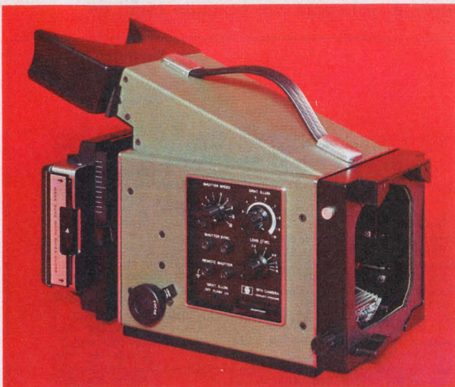
The HP 197A scope camera has a built-in UV light which can be used to record the black lines of internal-graticule scopes. The electronically controlled shutter of this Hewlett-Packard camera provides exposure times from 1/30 to 4 seconds.
