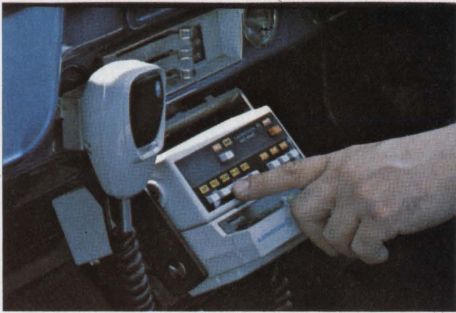
Status/message accessory from Motorola Communications enables mobile operator to send precoded digital messages back to base station.
