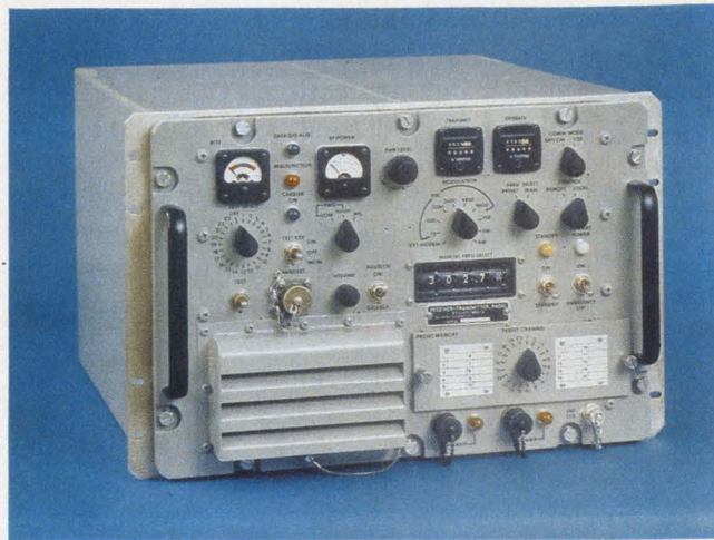
Tests of 23 key points in this 225-to-400-MHz Navy satellite communications terminal by Electronic Communications, can be made by nonskilled personnel operating a "Test-Select" switch.
