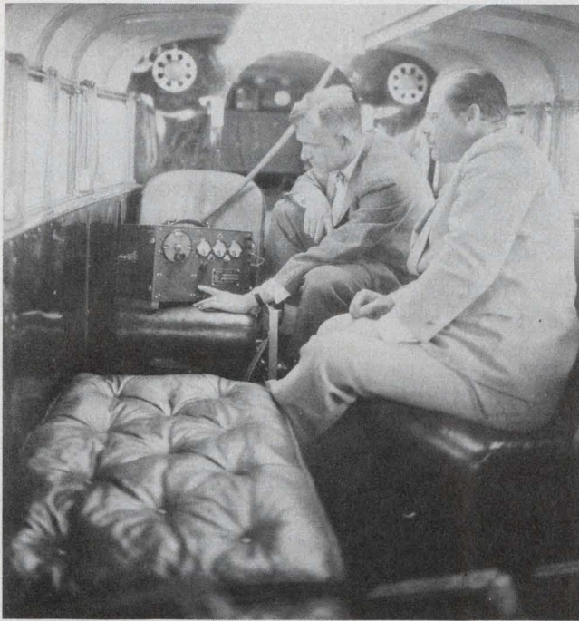
Dr. Alexanderson and S. P. Nixdorff examine one of Alexanderson's inventions—the radio-echo altimeter.
