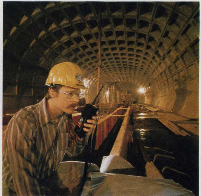
RCA's Tactec, a portable two-way radio, is used by subway construction worker in Washington, DC. These units provide up to 5-W output.
