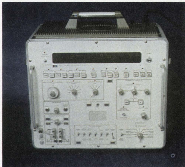
Multipurpose test instruments , such as this HP4940A test set, can provide a comprehensive analysis of an analog channel's characteristics without the need for additional equipment.
