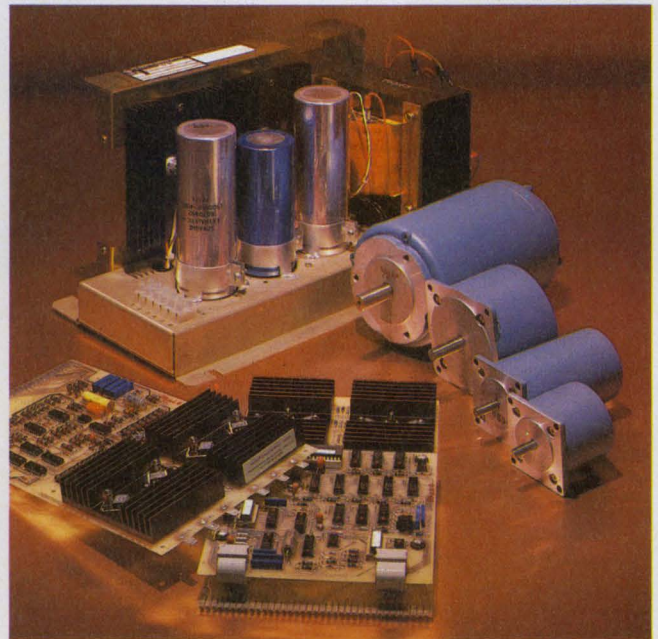
A stepper motor should be considered a system , not just a component. Electronic driving circuitry is needed and can significantly affect performance.
