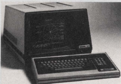
With built-in routines, the Tektronix 4025 creates pie or bar charts in a few seconds.
