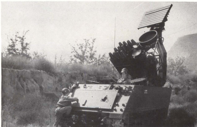
RADAR-GUIDED Mauler missiles will be used by Army to protect forward battle positions against bombing and strafing aircraft and short-range ballistic missiles and rockets. Maulers will be fired from moving vehicles. Photo shows engineering mockup of system, being developed by General Dynamics/Pomona; $16.6 million was just added to R & D contract.
