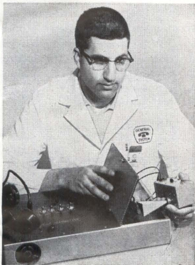
EMPHASIS on portability was demonstrated in Sylvania's new millimeter-wave communications set. Radiations from internal horn antenna produce a beam
