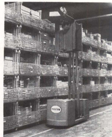
ORDER-PICKER takes high road while truck follows guide path on warehouse floor
