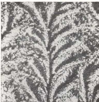
APPLIED ELECTRIC d - c field causes dendritic growth in silver telluride thin film. Recrystallization process is illustrated at left. Effect of a - c field on silver telluride growth is shown at right. From paper presented by C. Paparoditis of C.N.R.S. Laboratories, Bellevue, France, at single-crystal thin-film conference at Philco Research Center, Blue Bell, Pa.
