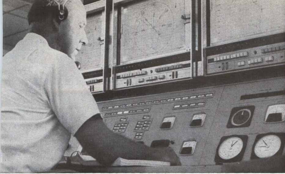
CONTROL CONSOLE at Eleuthera central station directs Mistram site and hand-over to Valkaria. Plotters show missile trajectory and position
