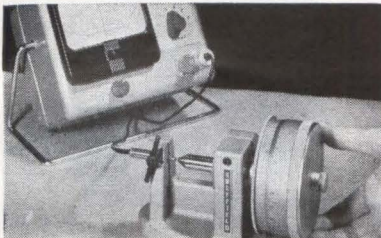
MICROMETER instrument weighs 6 pounds and measures 5½ by 6½ inches
