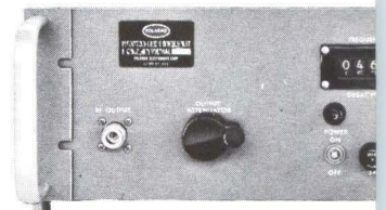
MODULAR SIGNAL SOURCE 1207 Freq. Range: 3.8 GC-8.2 GC
