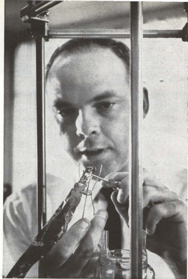
FOIL LEAD from modulation equipment is being attached to injection laser. Top of dewar for liquid nitrogen cooling is at bottom
