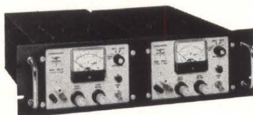
Two Trygon HR20-1.5's, rack-mounted side by side.
