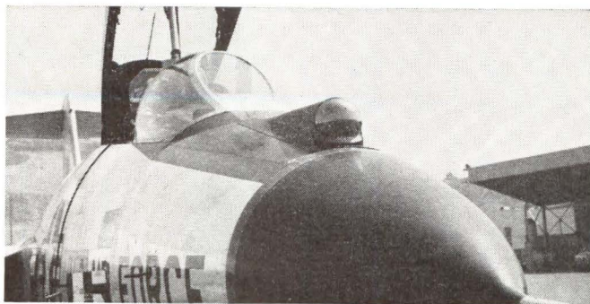
Interceptor IR installation
