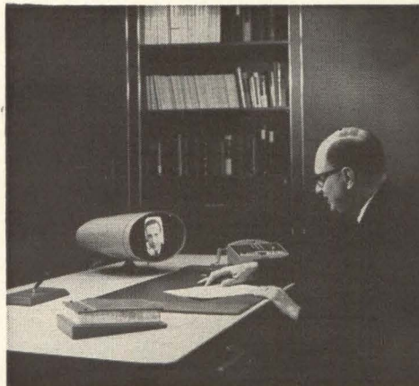
Larned Meacham , Bell Labs engineer and inventor who helped develop the latest visual telephone system at Holmdel, N.J., talks with Arthur Hall at Murray Hill, N.J. laboratories. In 1927 picture telephone tests, mechanical scanner at left sent picture-element signals to a screen in which 50 neon lamps were combined with a shutter to produce a crude halftone.
