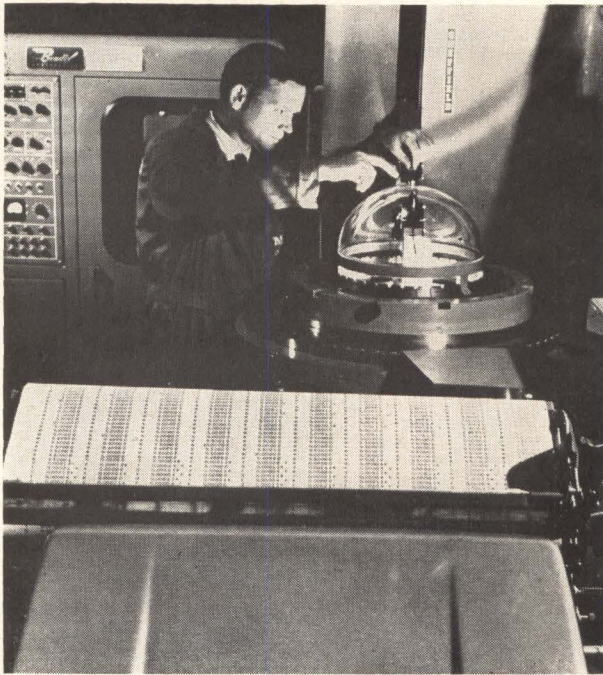
Millionths-of-an-inch deviations on the transparent part are automatically measured and recorded with this Sheffield six-coordinate inspection machine. Two probes measure simultaneously, one within the hemisphere and the other on the outside surface.
