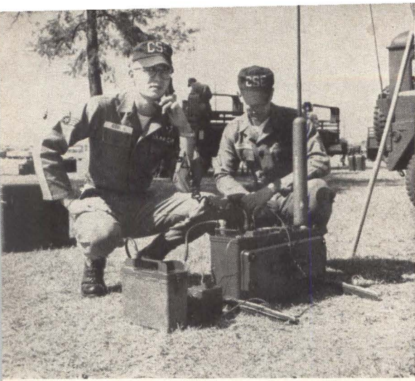
This 40-pound manpack radio was dropped at Delawar, and quickly put into operation by two men. Composed of two packages—a transceiver and a battery power supply and antenna—the AN/PRC-47 is single sideband, operates at from 2 to 12 Mc, provides 10,000 channels at one-hilo-cycle increments. It is used to start operating fast, before the bigger AN/TSC-15 is set up.
