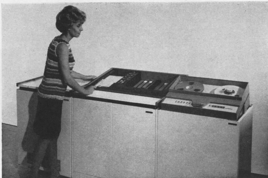
The Ampex CTS-2000 transfers computer data from 2,000 tab cards to magnetic tape in one minute.
