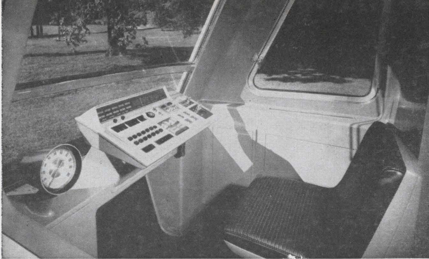
Interior of detachable pod at front of BARTD train. One man sits here to take control in case of emergency. With the control panel the crewman monitors the electronic control equipment on board; through the large front window he watches for fallen boulders and other track obstructions. He won't have to watch for people or for stalled cars; the track is completely fenced and there will be no grade crossings.
