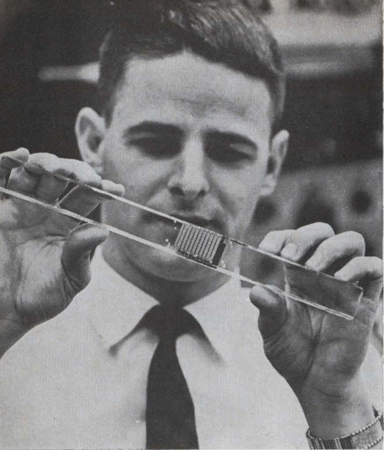
See-through. Anthony van den Heuvel, a scientist at IIT Research Institute, examines an acoustic delay line in which piezoelectric thin film taps are deposited on a glass substrate.
