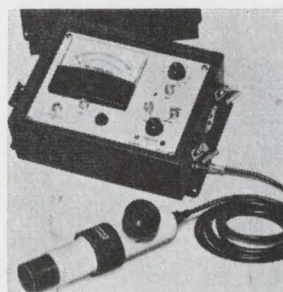
Infrared radiation pyrometer/controller called Industrial Pacemaker permits sensing the temperature of a workpiece or material in process of fabrication, without touching it. It covers the temperature range 1000^\circ to over 4000^\circ F with several convenient models. Unit is housed in a vapor tight cabinet for severe environments Irtronics Inc., 57 Commerce Road, Stamford, Conn. [387]
