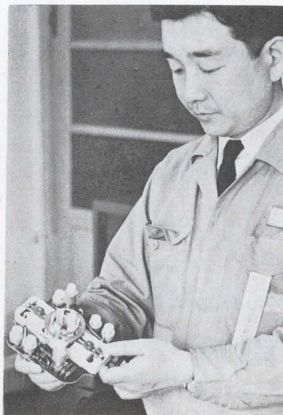
All there. Simplified convergence circuit mounts on a single board that fits on neck of picture tube.
