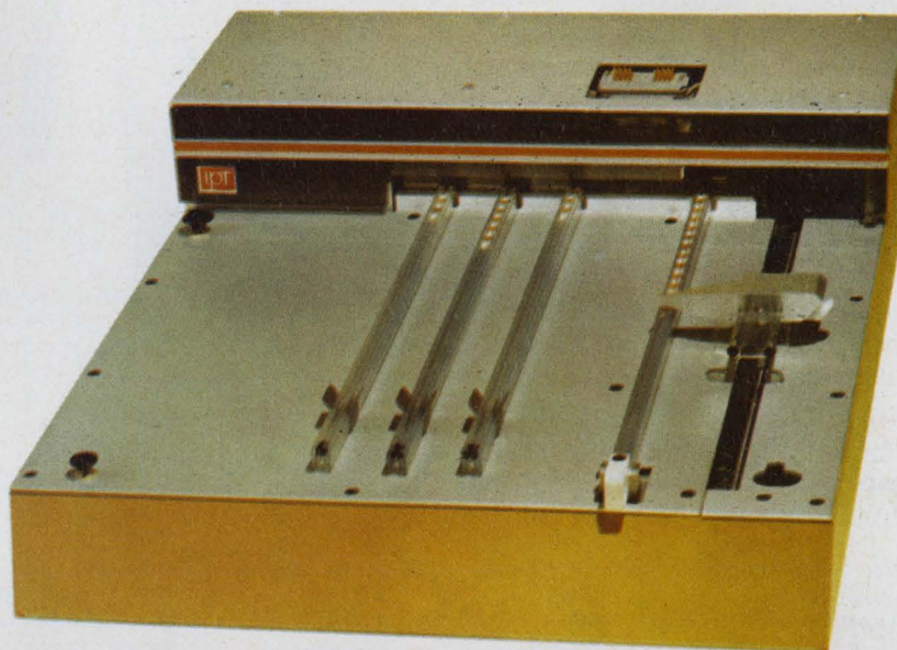
Positive feed. Finger at right pushes devices toward the test heads at back part of handler. Three output sticks at left hold tested circuits that have been sorted into performance categories.
