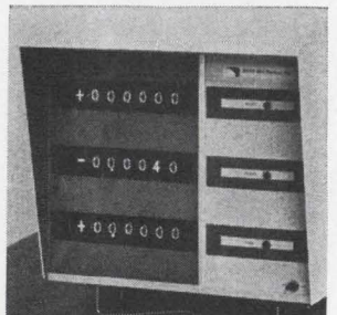
Bidirectional counters come in single- and multi-axis units. Featuring all-TTL integrated circuitry on plug-in IC cards, they offer high noise immunity for industrial environments and high-speed capability as well. Applications include position or speed measurement and control for machines, and numerical and process control systems. Data Technology Inc., Watertown, Mass. [408]
