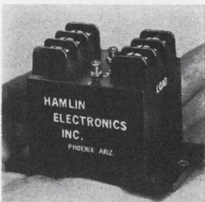
A-c controller is designed for 3-phase, fractional h-p motors, and was developed primarily for the computer peripheral device market. It provides arcless make and zero current break. These attributes reduce rfi and emi to levels where equipment drive motors can be operated adjacent to low level logic circuits. Hamlin Electronics, 3879 N. 28th Ave., Phoenix 85017 [405]
