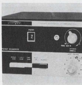
Ten point scanner model 634 is used to sequentially transfer analog data from multiple sources to one measuring instrument. Scanning is accomplished by two-pole reed relays suitable for switching low level sources, such as thermocouples. Dwell time on each point is adjustable by front panel control. Price is $575. United Systems Corp., 918 Woodley Rd., Dayton, Ohio 45403 [362]
