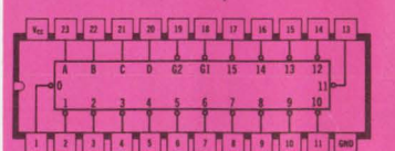
SN54/7448 BCD-to-7-Segment Decoder/Driver
