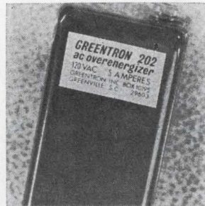
Modular solid state over-energizer applies full a-c line voltage to the load for one second. The load voltage then drops to a lower, adjustable level. This level is maintained until power is shut off. Unit recycles automatically when power is applied. Steady state rating is 5 amps. Price is $16; delivery, stock to 4 weeks. Greentron Inc., Box 10195, Greenville, S.C. 29601 [402]
