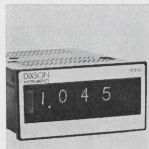
Frequency counter-tachometer FT300 is a four-digit panel meter that has five easily changeable frequency ranges and two tachometer ranges with maximums of 1 Mhz and 100,000 rpm, respectively. Features include adjustable display time, overrange indicator, input sensitivity adjustable from 50 mv, and 1-megohm input impedance. Dixon Inc., Box 1449, Grand Junction, Colo. [3671]
