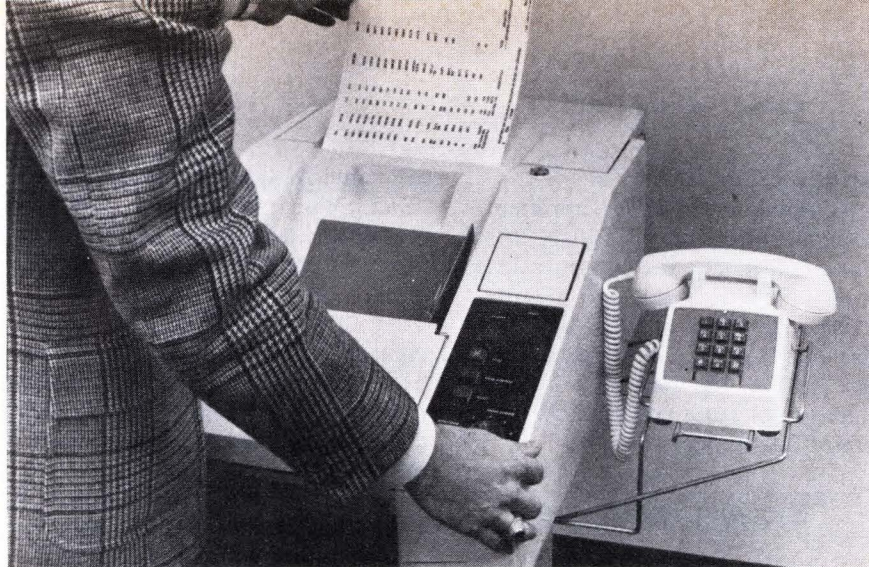
Plain fax. A helium-neon laser inside Xerox Corp.'s new two-minute facsimile machine creates images on plain paper, using the company's xerographic process.
