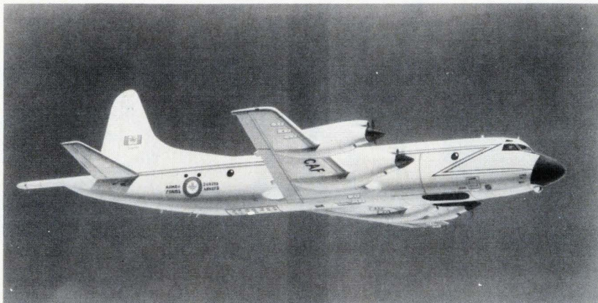
New combo. CP-140 bought by Canada for submarine surveillance combines Lockheed-California Co.'s P-3 Orion airframe with avionics developed for the carrier-based S-3A Viking sub hunter. Canada also plans to use the craft for detecting forest fires.
