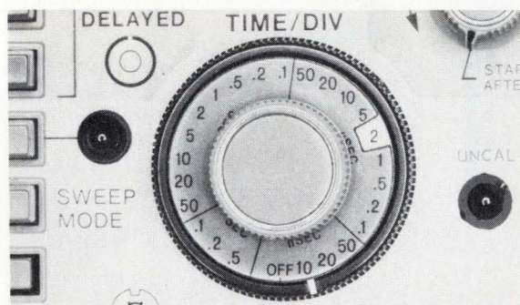
3. Checking the time base scale-factor
