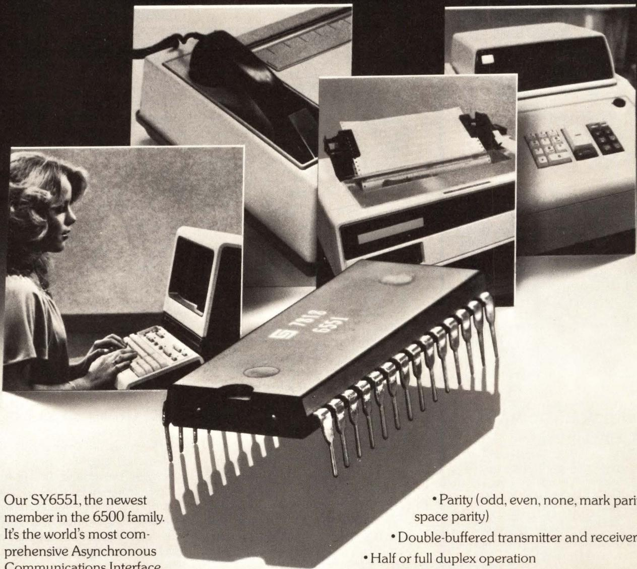
Our SY6551, the newest member in the 6500 family. It's the world's most comprehensive Asynchronous Communications Interface Adapter. Here's why: on-chip programmable baud rate generator... 15 programmable rates up to 19.2 kilobaud... small size because we've not penalized the asynchronous communications user with unneeded synchronous protocols & conventions... full compatibility with both 6500 and 6800 microprocessors... and all it requires is a single +5V power supply.
