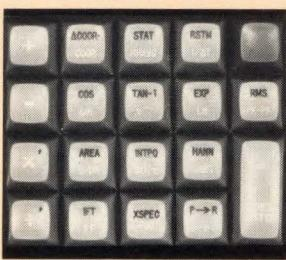
**TIME DOMAIN PROCESSING** — Pre-programmed keys convert to engineering units, integrate, differentiate,  $+$ ,  $-$ ,  $*$ ,  $\div$ , perform statistical investigations, measure RMS, Rise-time,  $1/\Delta T$ , etc.
