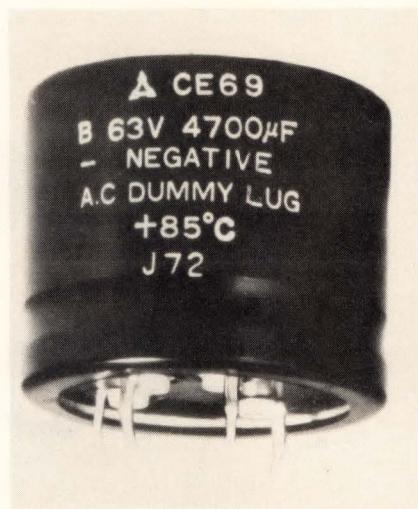
electrolytic capacitors, on the other hand, do not impose such design constraints: their body height is less than or equal to their body diameter.
