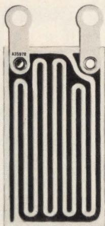
temperature range of  $-60^{\circ}\text{F}$  to  $+200^{\circ}\text{F}$ . Response time is largely a function of ventilation. At zero ventilation, the transducer takes at least 30 seconds to register a 63% change in relative humidity; this drops to milliseconds with moderate air ventilation.
