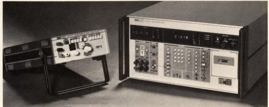
515A meter calibrator and the 5101A "cal lab in a box."
