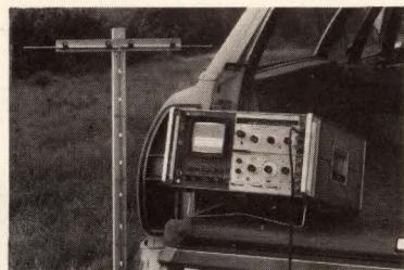
Use the 8554B tuning section to cover the 100 kHz to 1250 MHz range. Maximum resolution is 100 Hz. Measure with  $\pm 1\frac{1}{4}$  dB accuracy. Its companion HP 8444A Tracking Generator (500 kHz to 1300 MHz) also works with the 8555A tuning section.
