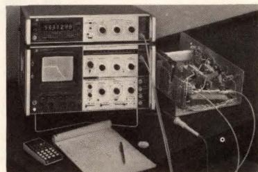
The 8553B takes you from 1 kHz to 110 MHz with  $-140$  dBm sensitivity and resolution as high as 10 Hz. Signals can be measured with  $\pm 1\frac{1}{4}$  dB accuracy. Choose the companion HP 8443A Tracking Generator/Counter for wide dynamic range swept frequency measurements and precise frequency counting.
