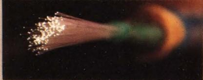
Optical communication cables are being used in computers, process instruments and control applications. They weigh less and take less space. They eliminate electrical and electronic interference as well as ground loops. They can be more economical. And every day, they're making the old standard interconnect systems obsolete, one by one.
