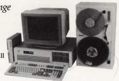
With 9-track tape, you are free to exchange data files with any mainframe or minicomputer in the world.
