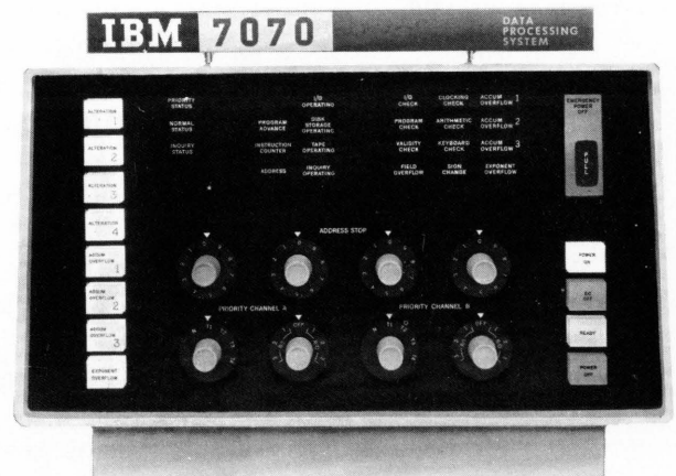
FIGURE 2.3-1 OPERATOR'S CONSOLE SWITCH AND LIGHT PANEL
