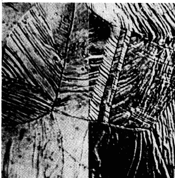
Figure 5 Cold-worked bronze (1000 \times ).
