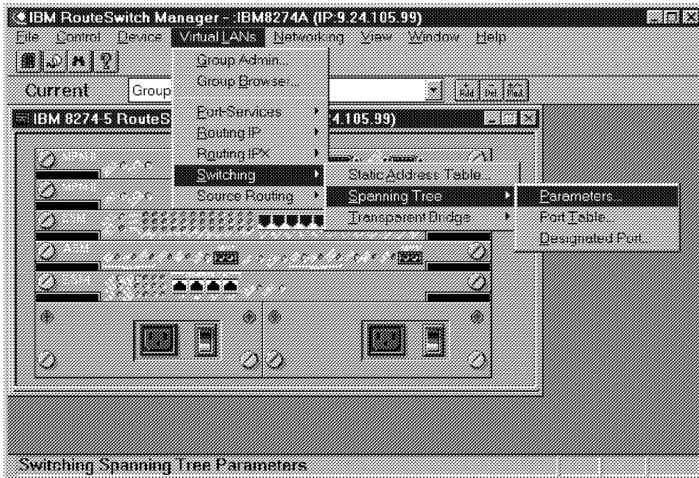
Figure 76. Selecting Spanning Tree Parameters from RouteSwitch Manager
