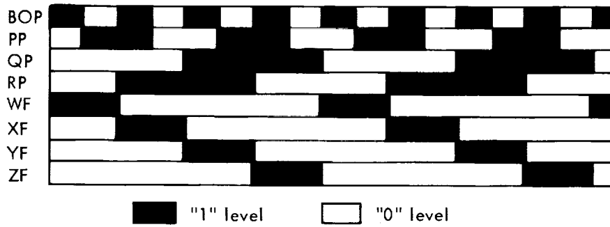
Figure 2-14. Clock Generator Timing
