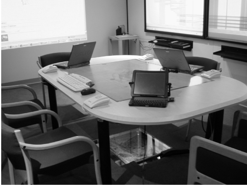
Figure 3 - The iTable, a bottom projected table used to experiment with table top UIs
