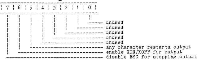
When set, "Any Character Restarts Output" bit instructs the terminal drivers to restart the output if it has been stopped by either an escape or XOFF.
