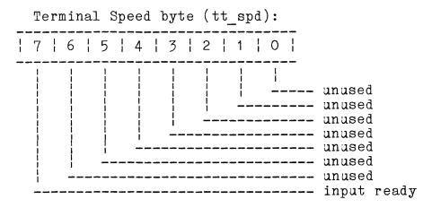
Under normal input operations, the "Input Ready" bit is not set until an entire line has been input and terminated by a carriage return. There are special input modes which can be established, however, where the "Input Ready" bit will be set as soon as a single character is input. These are the "raw I/O mode" and the "single character input mode", and are described later in this section.
