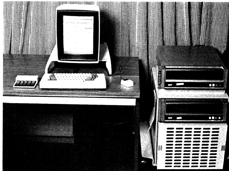
Figure 4.1. Picture of typical Alto work-station with keyset, screen, keyboard, mouse, computer with two disk drives.
