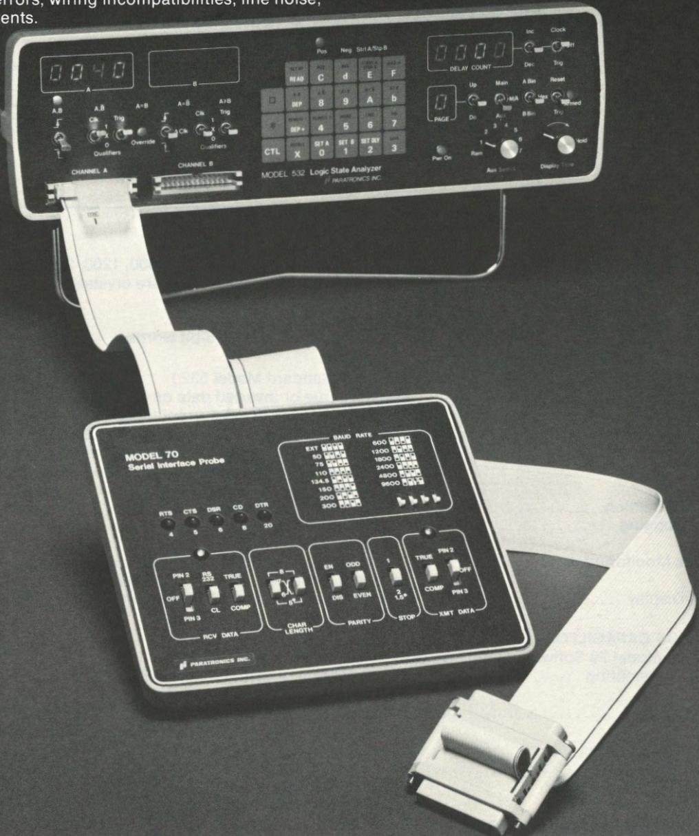
The Model 70 Serial Interface Probe converts the Model 532 Intelligent Logic Analyzer into a powerful tool for testing asynchronous RS-232, CCITT V.24, and 20 mA current loop interfaces.
