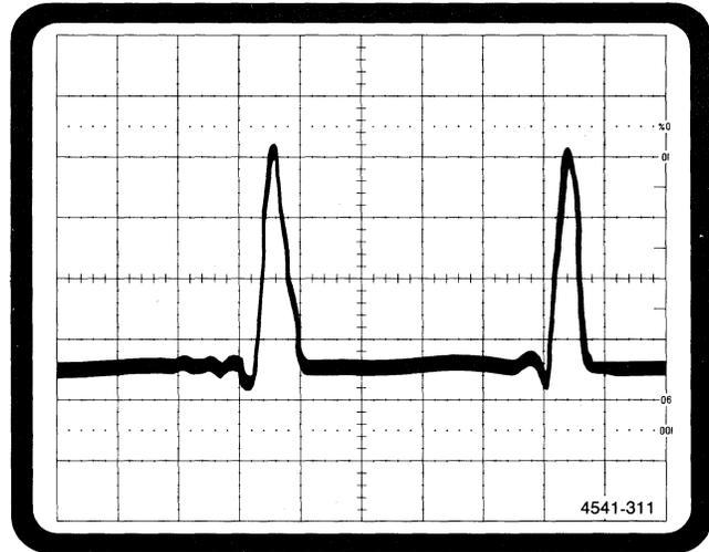
Figure 5-29. 50 MHz pulse generator waveform.
