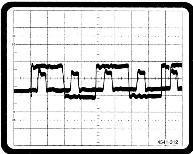
Figure 5-30. 100 MHz oscilloscope waveform for step 5 of the performance check (time base = 50 ns).
